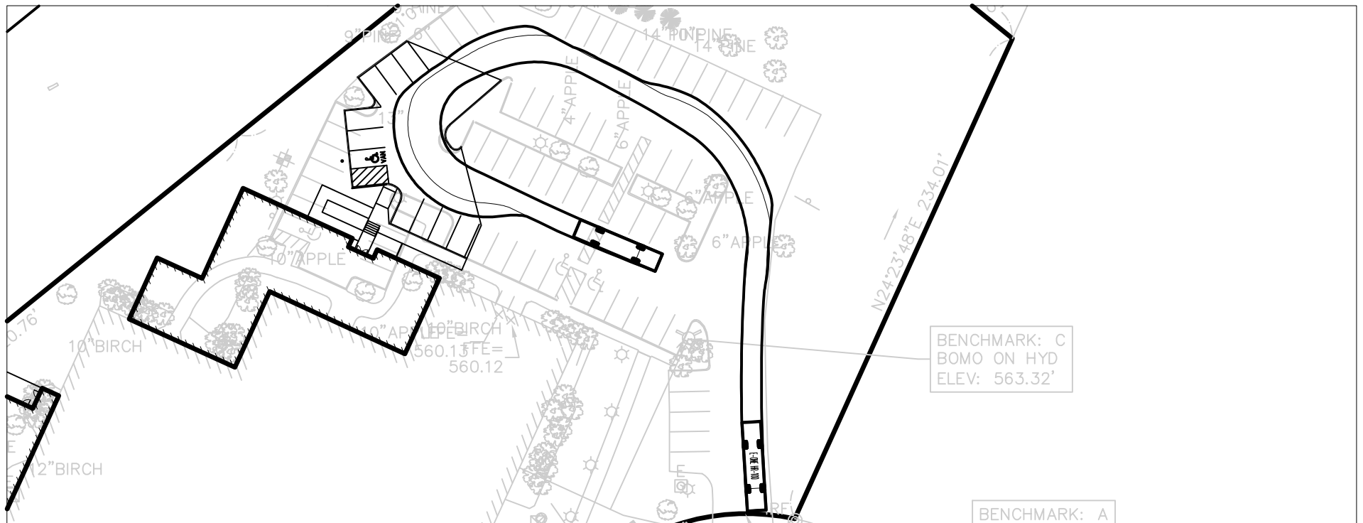
FIGURE 2 – E-ONE HR-100 FIRE TRUCK TURNING INTO NORTHERN PARKING
