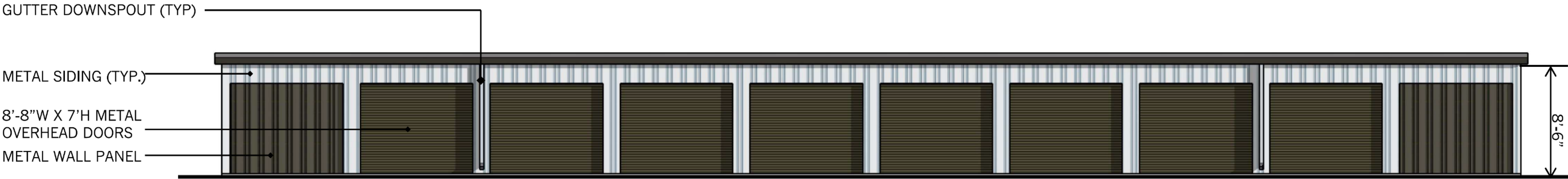
TYPICAL STORAGE BUILDING FRONT & REAR ELEVATION
