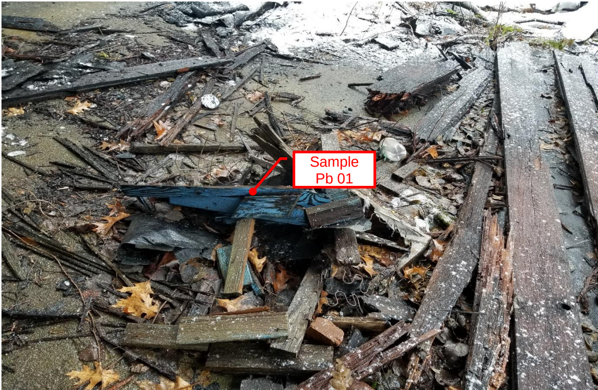
Photograph 8: Round House – Wood Debris on Floor. Blue Paint Chips (Lead, 1.34 mg/Kg, 1 CY - 2 Debris Piles)
