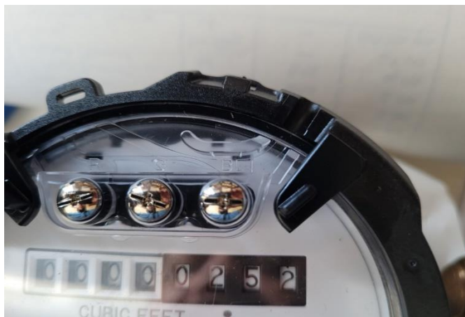
An example of a register on a meter displaying a meter reading. This is a meter one inch or smaller.
