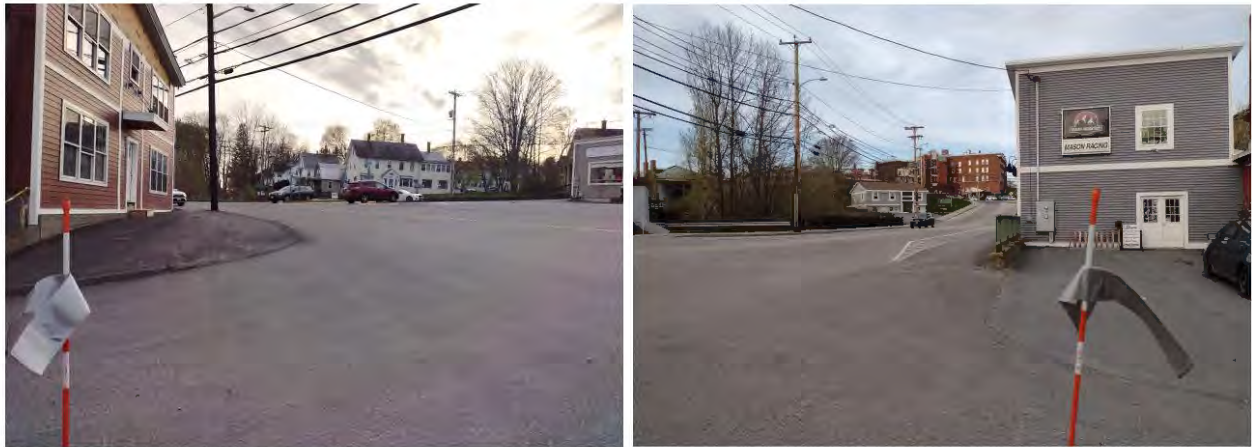
FIGURE 5: DRIVER'S PERSPECTIVE 15-FEET FROM THE EDGE OF TRAVEL WAY AT FOUNDRY STREET TO THE WEST (LEFT) AND EAST (RIGHT)
