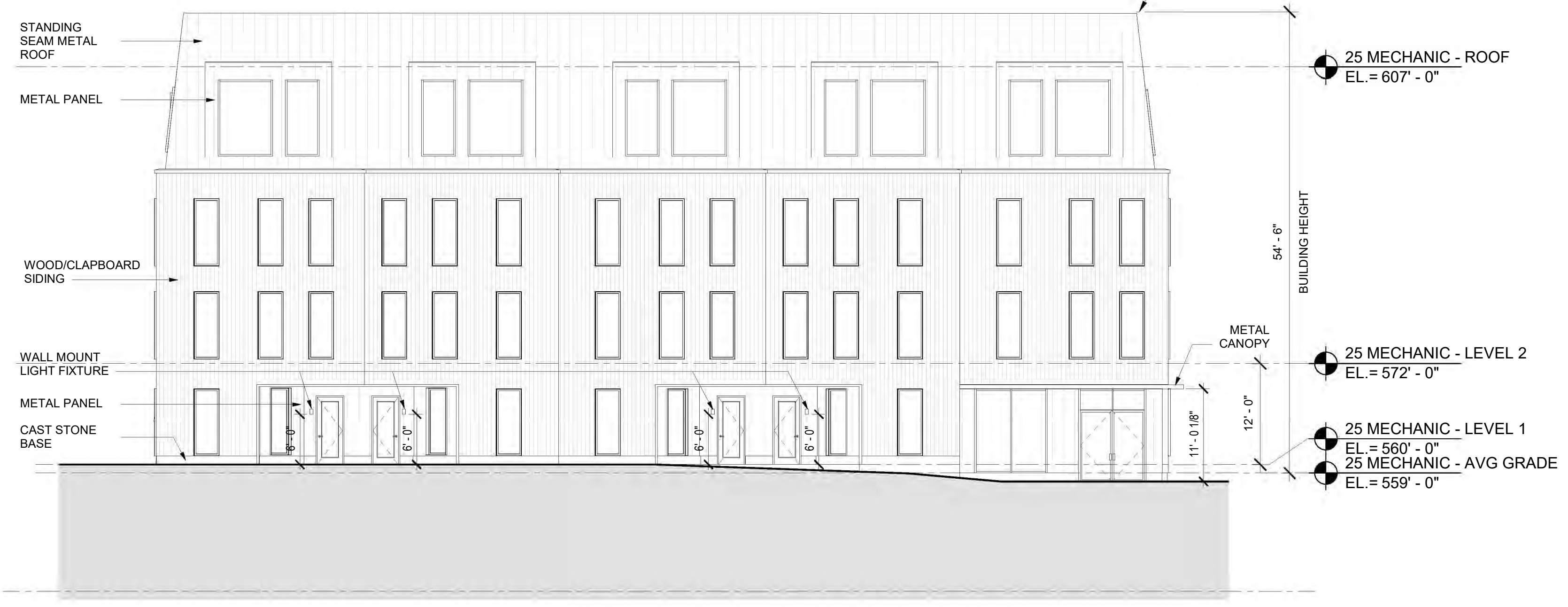
1 25 MECHANIC - WEST ELEVATION 3/32" = 1'-0"
