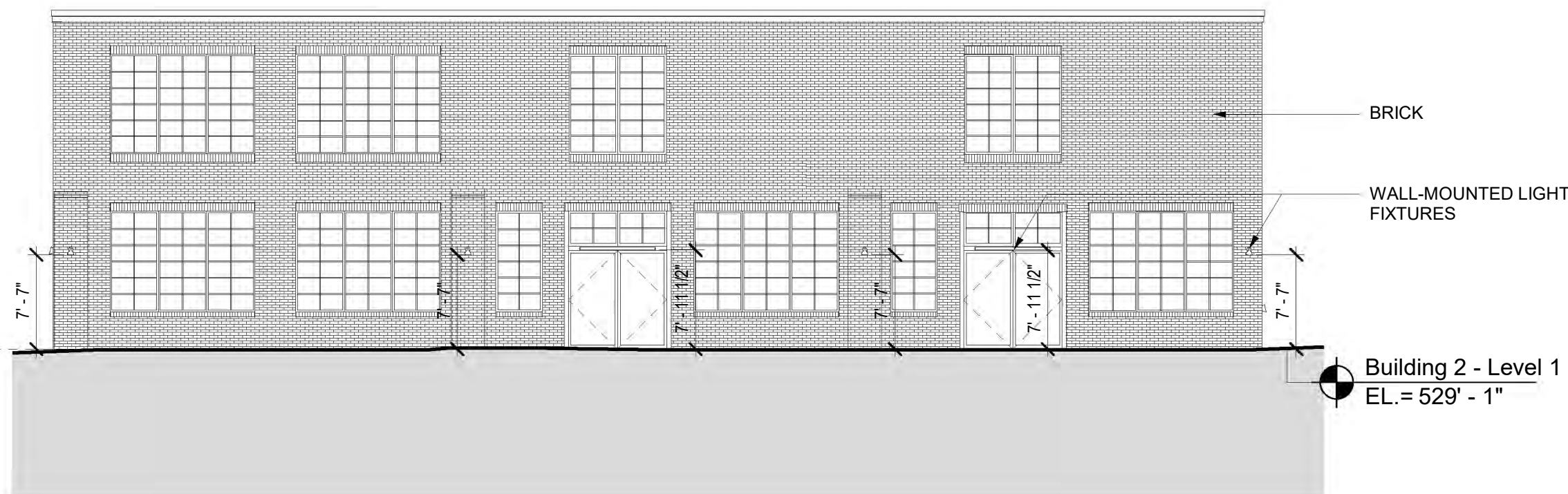
1 BUILDING 2 - EAST ELEVATION 3/32" = 1'-0"
