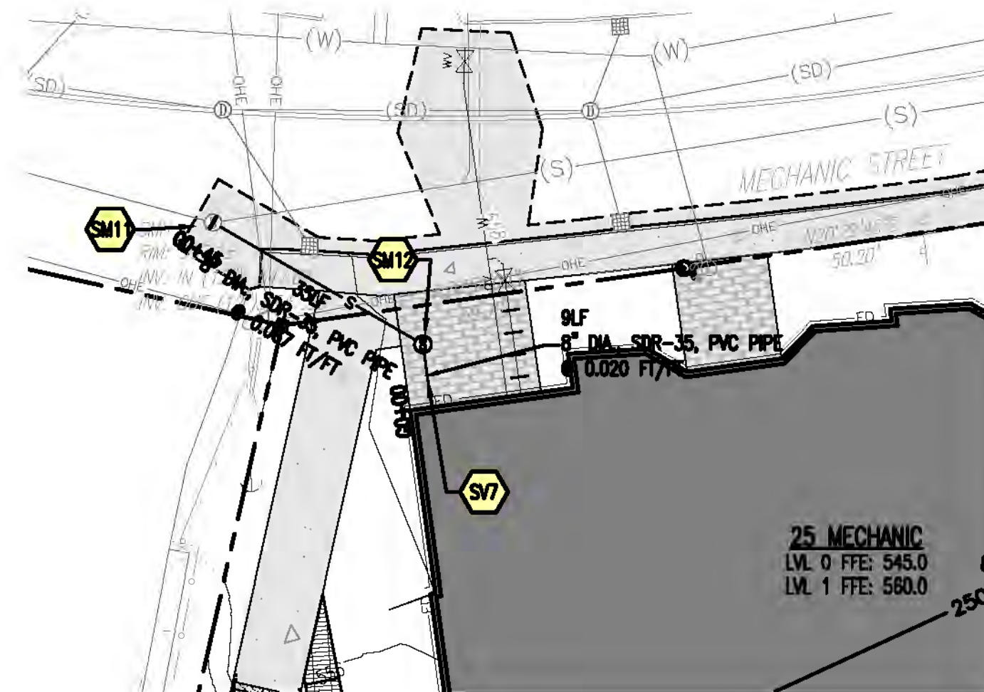
SEWER ALIGNMENT "G", STA 0+00 - 0+44.74
