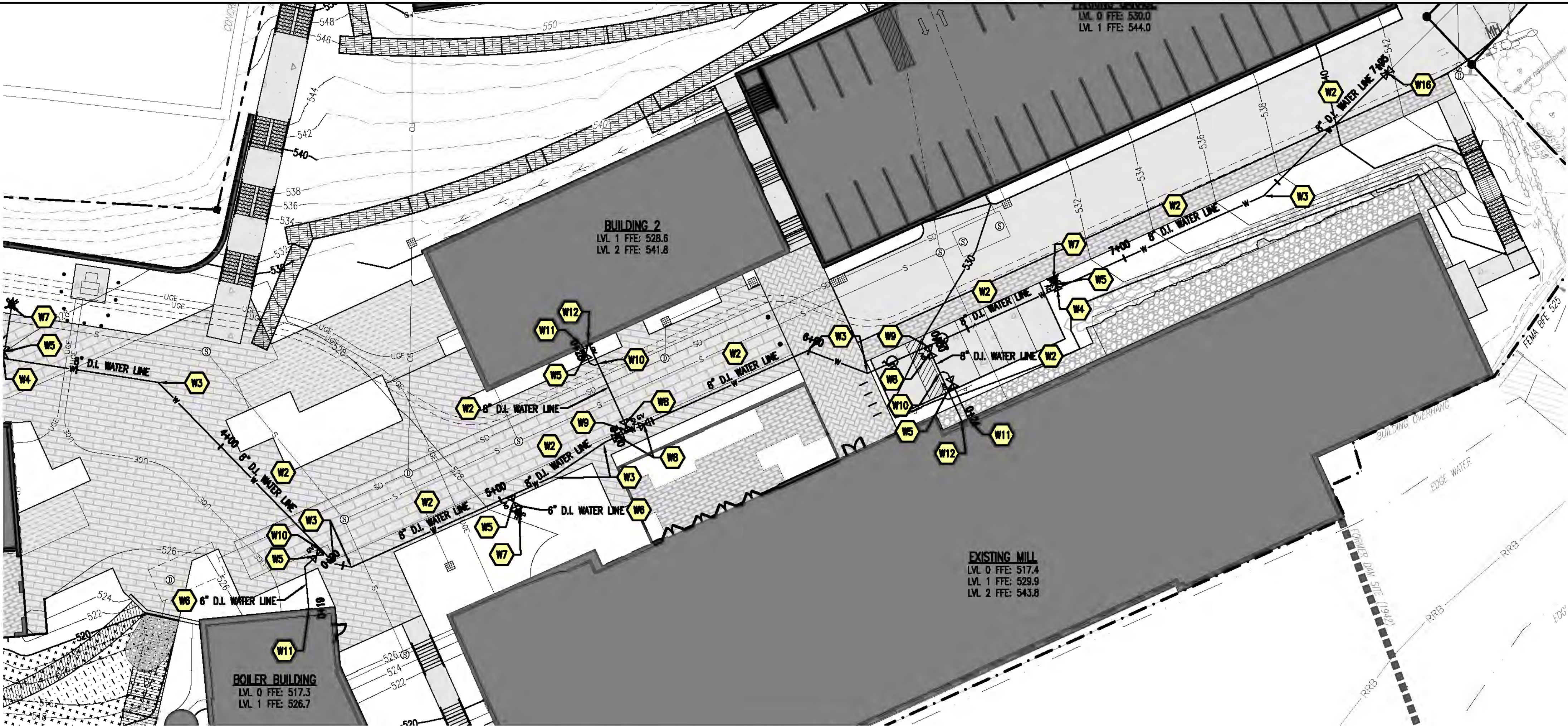
WATER LINE PLAN VIEW – ALIGNMENT "A", STA. 4+00 – 7+95
