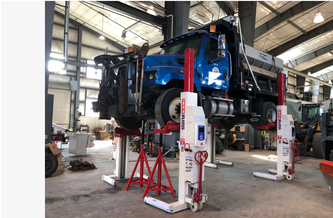
Demonstration of Mobile Lifts at DPW Garage
