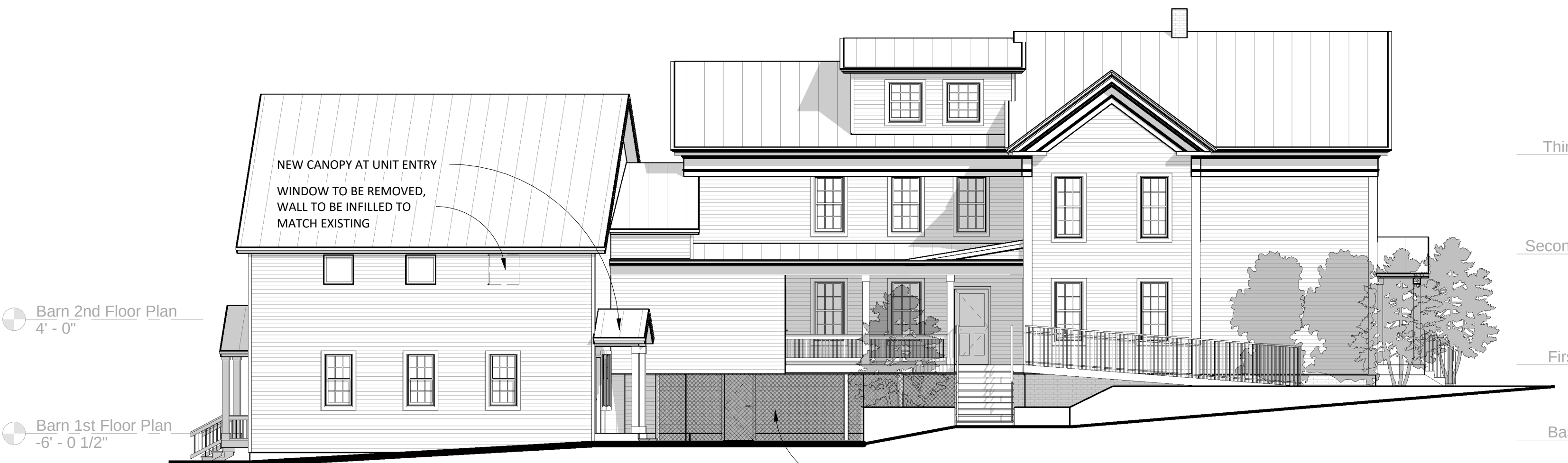
② West elevation - SPR 1/8" = 1'-0"
