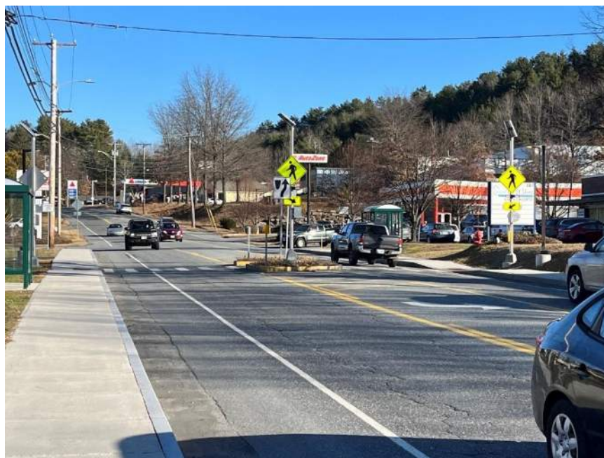
Figure 2 - Crosswalk with Median Refuge Island
