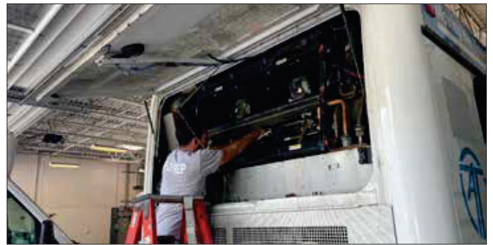
Air purification system installation in July 2022
