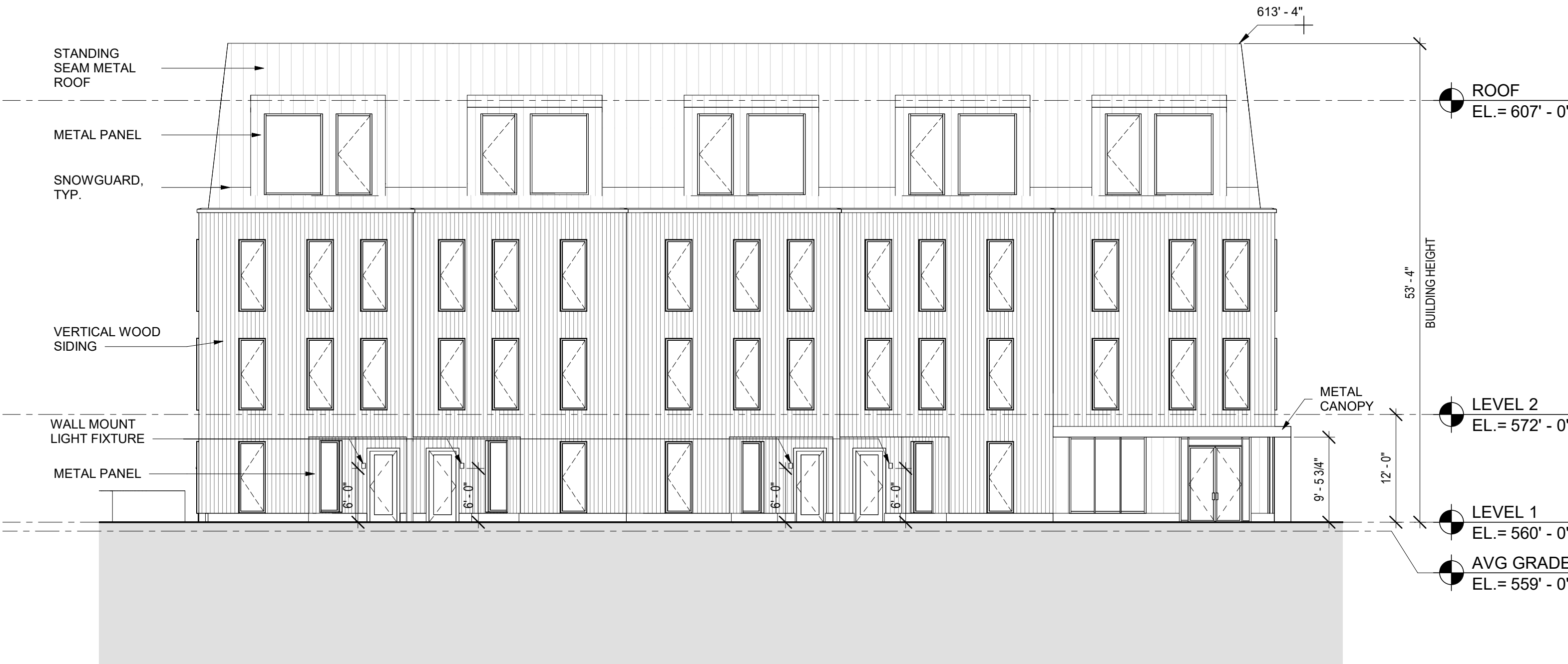
1 SPR - 25 MECHANIC - WEST ELEVATION 3/32" = 1'-0"
