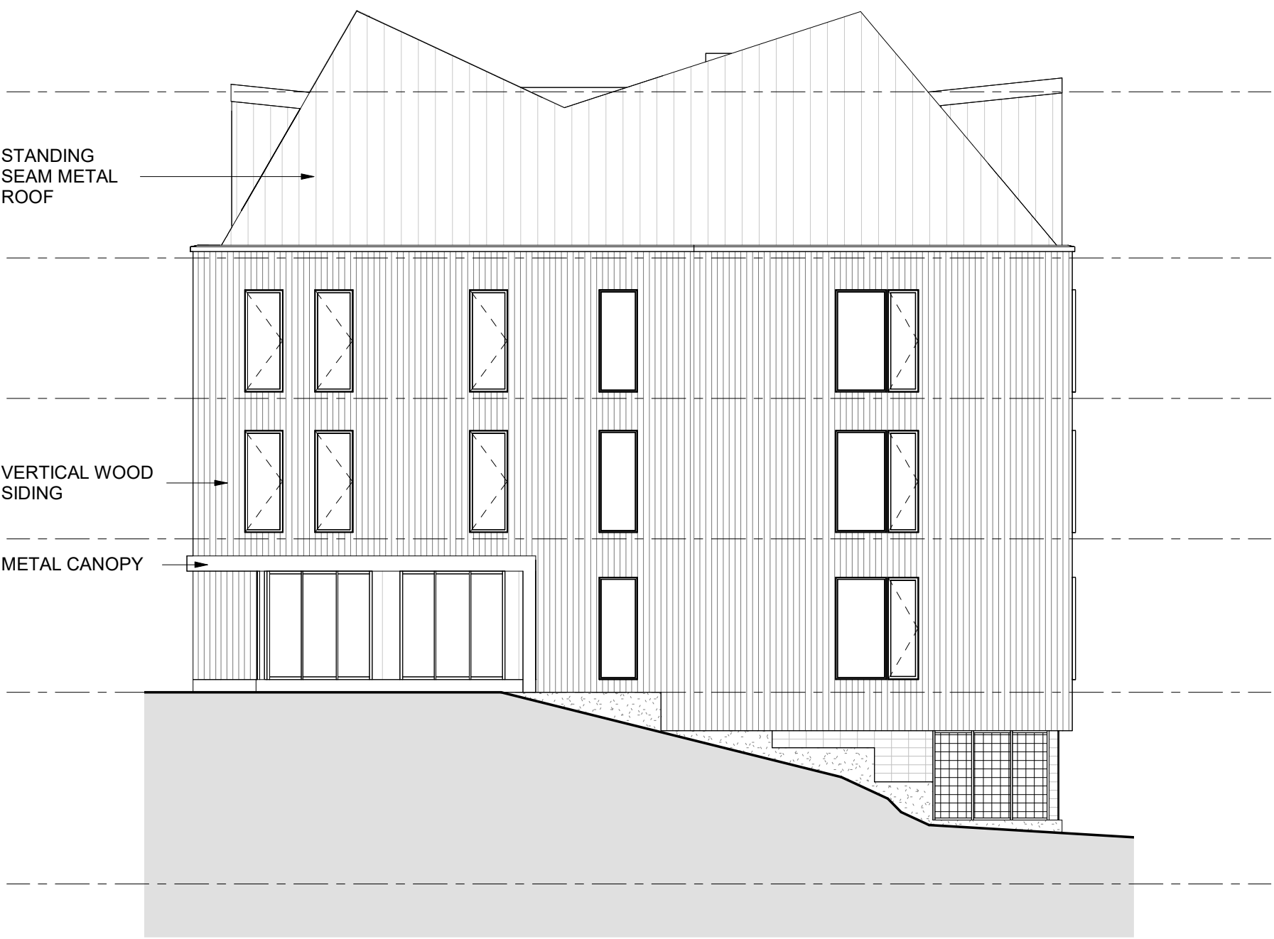
4 SPR - 25 MECHANIC - SOUTH ELEVATION 3/32" = 1'-0"
