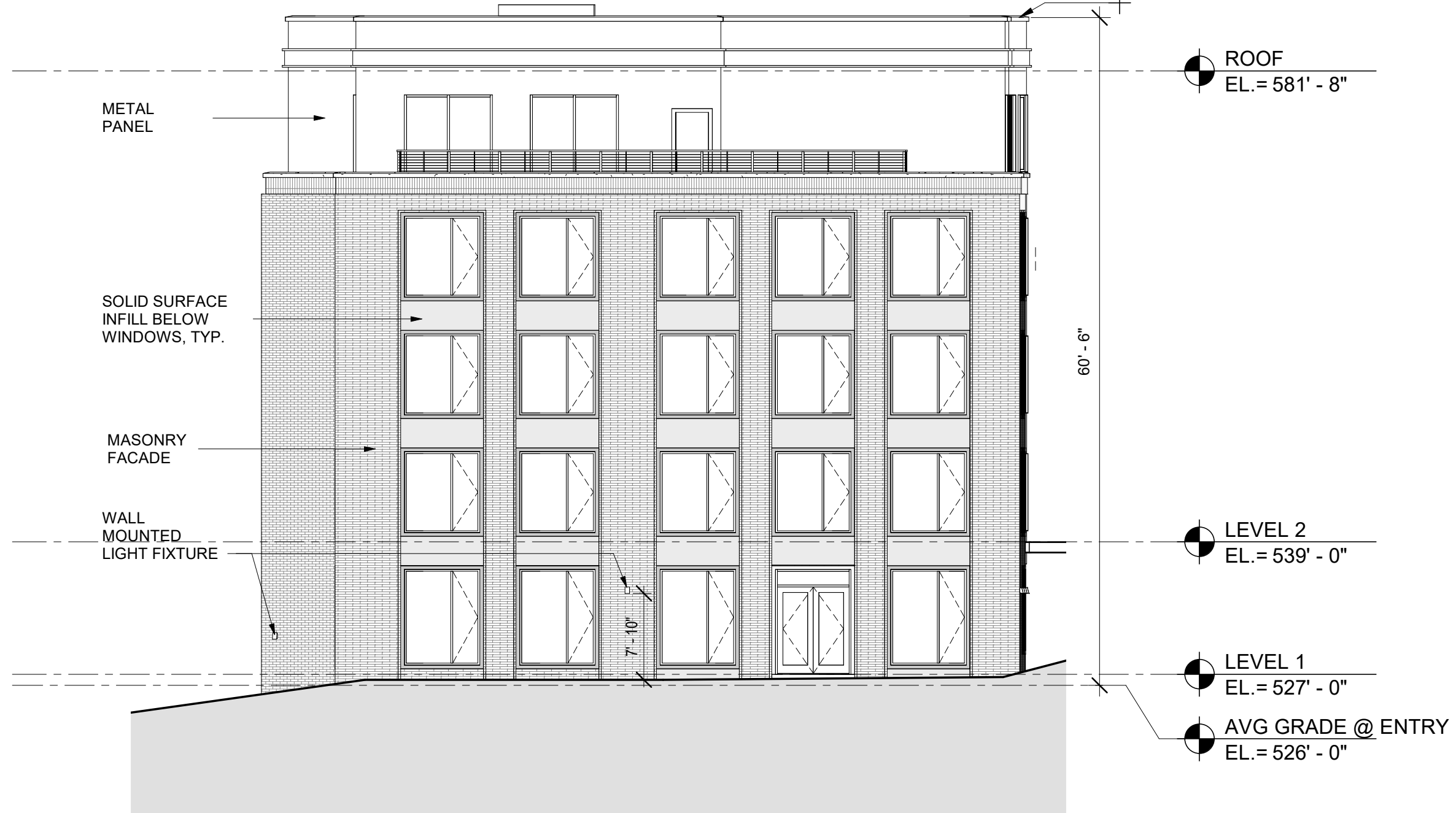
1 BUILDING 3 - NORTH ELEVATION 3/32" = 1'-0"
