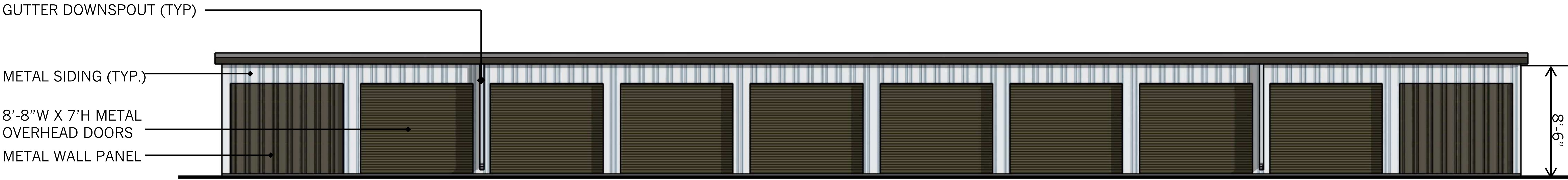
TYPICAL STORAGE BUILDING FRONT & REAR ELEVATION
