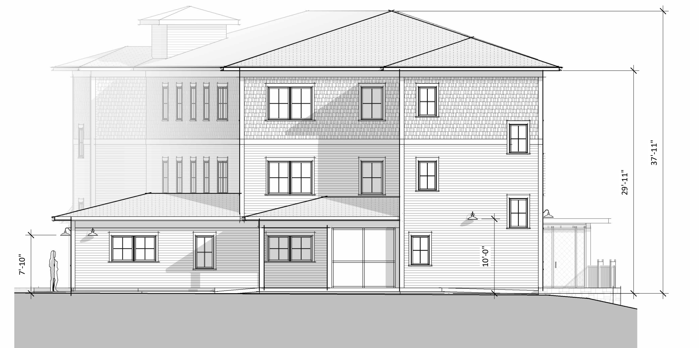
④ West Elevation (Front) 1/8" = 1'-0"
