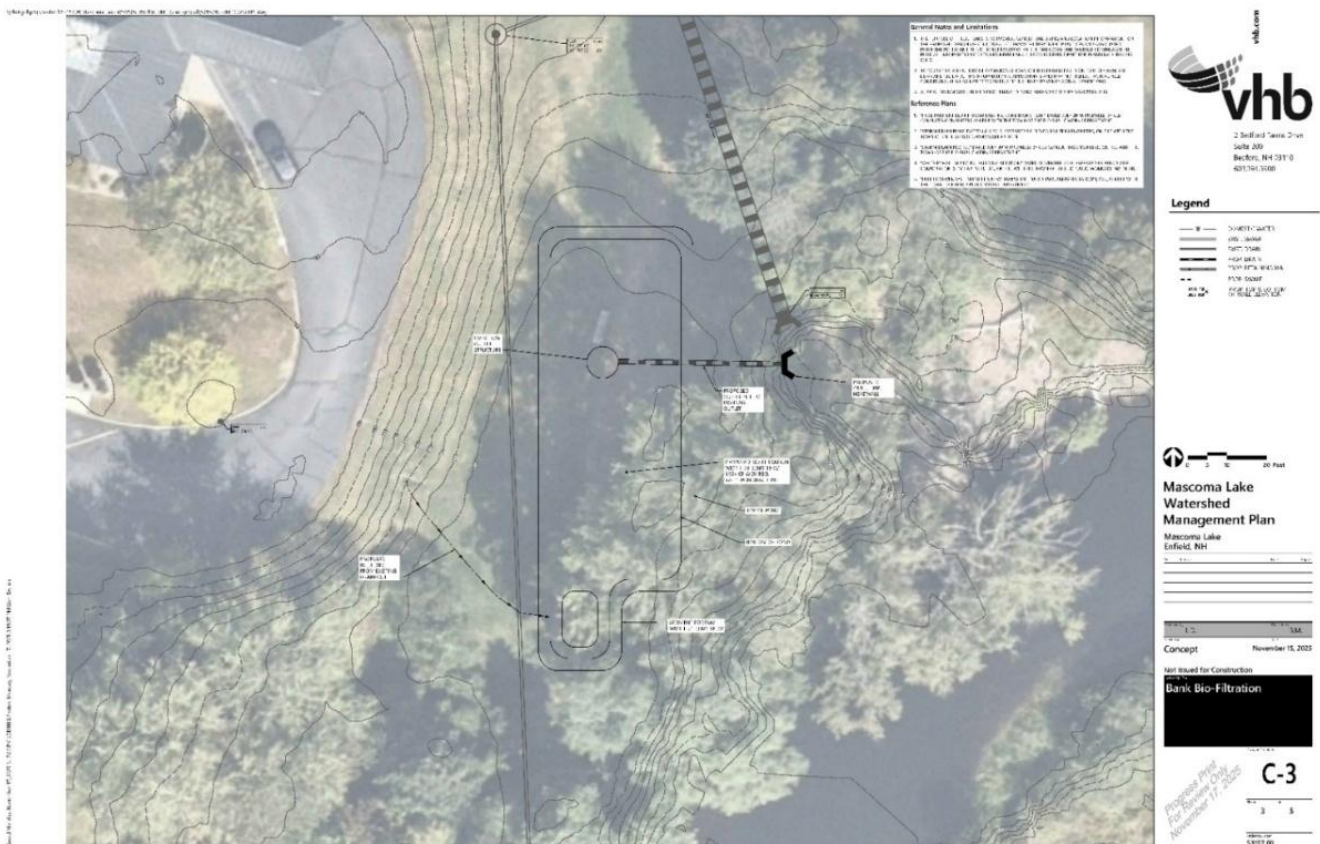
Figure 17. Site C-3 Mascoma Riverbank Biofiltration site plans by VHB. Refer to Appendix C: SCM Conceptual Site Plans for enlarged images.
