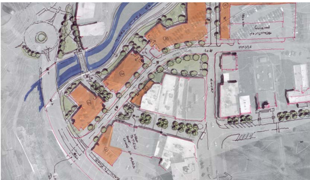
Figure 3.1 – Alternative 3 Tunnel Removal and Re-development Concept
